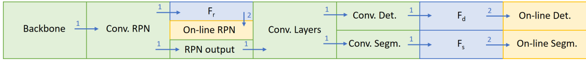
Figure 6.4 Ours training protocol. We rely on the feature extraction layers of Mask R-CNN pretrained on the FEATURE-TASK to simultaneously extract F_r , F_d and F_s . We then use these features to train the three on-line modules on the TARGET-TASK. The values on the arrows correspond to the training steps in Section 6.3.4.
