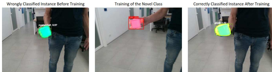
Figure 6.10 Dealing with false positives. Left image : an unknown object (a glass) is misclassified (as a masterchef ). Center : training. The robot is provided with the correct label and a demonstration of the object. Right : after training the new object is correctly classified.
